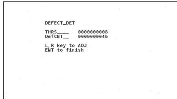
First, you will start off by completely blacking out the image on the camera (covering the camera lens, or blocking any light from hitting the lens)
