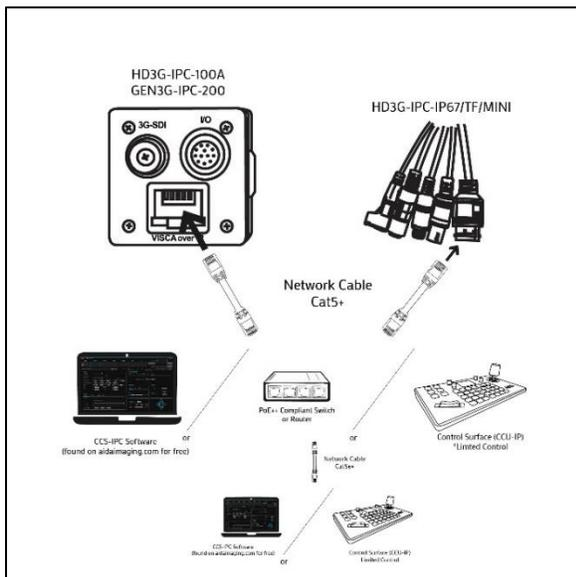
**1** You can directly connect a ethernet cable to the back of the camera, or pigtail of the camera to a computer, control surface, or switch/router to get VISCA over IP running. You could also connect
