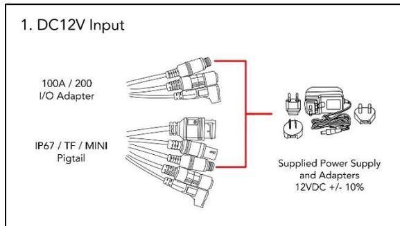
**1** Pick your preferred plug type out of the adapters securely fasten the end with the supplied factory adapter.
