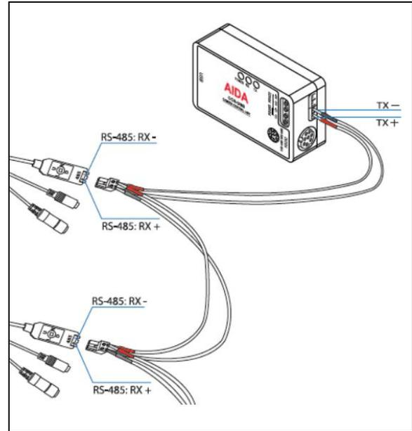
**3** Once connected, you can change the settings of the serial settings on the camera via the OSD menu, where you can find the baudrate, address ID, etc.
