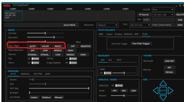
Once that is done, you can now control the camera using VISCA over IP. Do note that if you have multiple cameras, you will need to change the IP address of each camera to not conflict with one another. More will be mentioned in the networking section of the manual.
