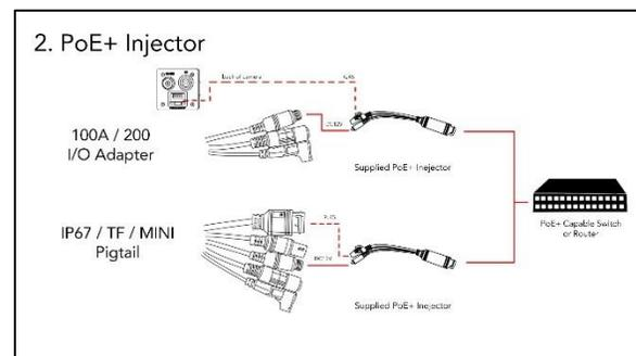
**1** Use a Cat5e or better patch cable to connect to a PoE+ compliant switch or router.
