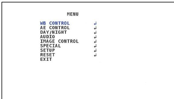
Using the joystick attached on the I/O cable, or pigtail of the camera, you can navigate through the menu using the U, D, L, R movements, and click of the joystick in neutral position.
