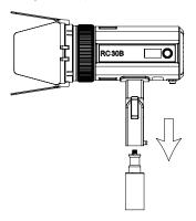
3. Insert the handle of umbrella softbox into into the hole and lock the knob.
